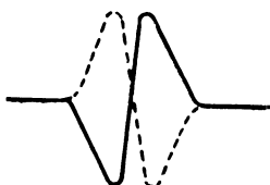
Fig. EE-80 Wave Form of Pick-Up Coil
