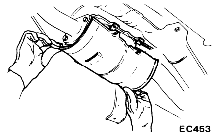
Fig. EC-67 Removing Catalytic Converter
